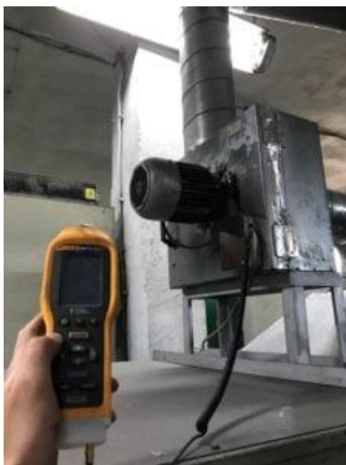
Figure 4. The vibration tester can use an external sensor to measure overall vibration values
