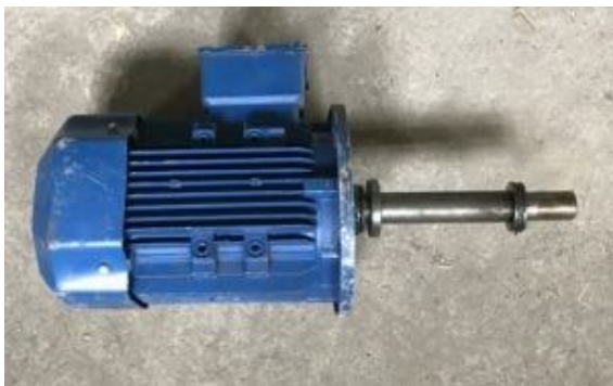
Figure 2. A shaft extender connects the motor to a fan
